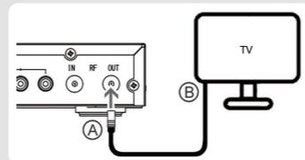
Connect as shown below by an antenna cable.
