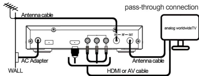
It is recommended that you connect the tuner and your analog TV as shown above. By this connection, you can watch
